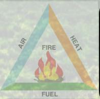
Fire needs three things to remain alight. Remove either the fuel (like wood, dried grass, hay), air (oxygen) or the heat (matches, flame) and the fire will go out.
